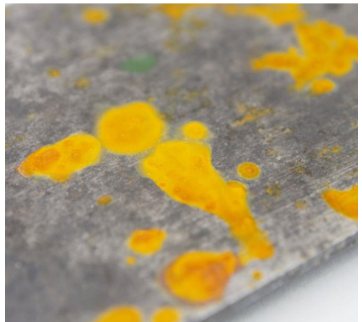
Figure 8: An example of flash rust after blast cleaning steel. Photo courtesy of Graco ( https://www.graco.com/us/en/contractor/solutions/articles/how-to-prevent-flash-rust-when-wet-blasting.html )
